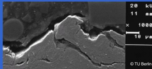
Cross section of a blast cleaned steel plate
